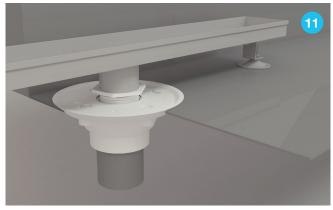
**Step 11.** Place the drain base into the threaded nipple. Use the adjustable feet to keep the drain channel into the correct position and level.
