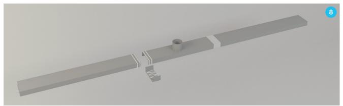
**Step 8.** Clean all parts. On a flat, stable surface, align the cut ends of the base with the outlet section. To join the base pieces to the outlet, attach joiner strips to the underside of the seams, using clear PVC primer and PVC cement.
